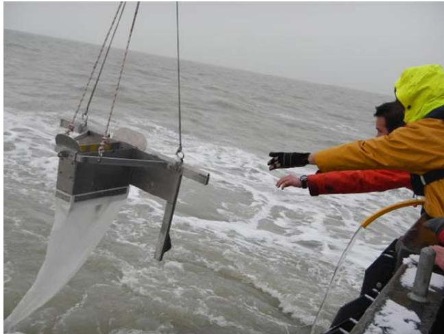
Photo: Microplastic sampling with a manta trawl. Crown Copyright 2013, permission granted by Thomas Maes, Cefas.
