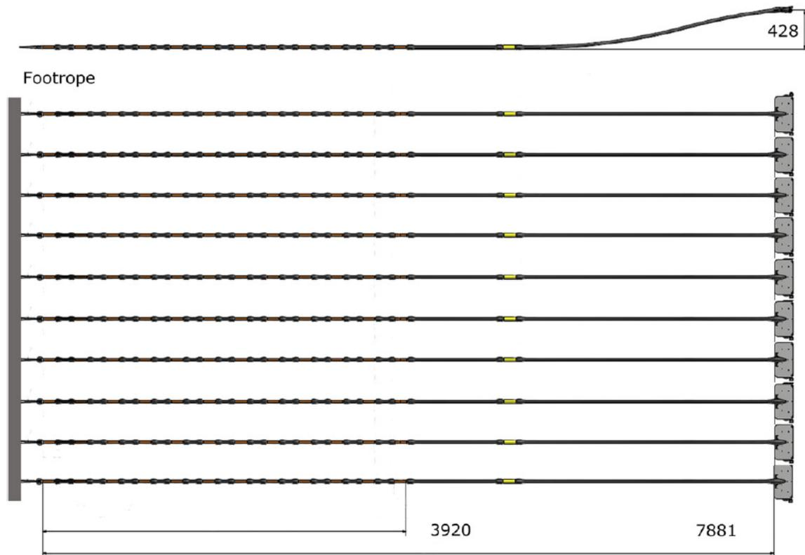
**Figure 2** Rigging of the electrodes of a 4 m pulse trawl used by Euro cutter vessels (221 kW). The bottom panel shows the top view of ten electrodes rigged between the wing and the groundrope. Each electrode consists of 12 conductor elements, evenly placed over a length of 3.92 m that are in contact with the seabed.
