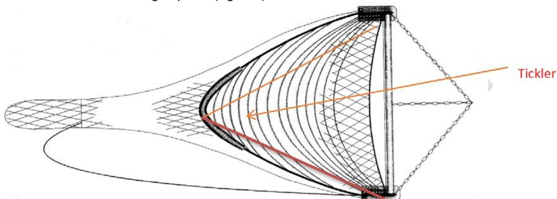
**Figure 1** Schematic of traditional beam trawl
